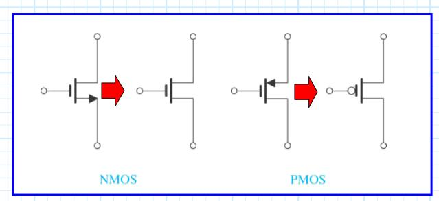
Effectively, these symbols represent the fact that we are now considering MOSFETs as switches, which can be placed either in an open state or a conducting state.
